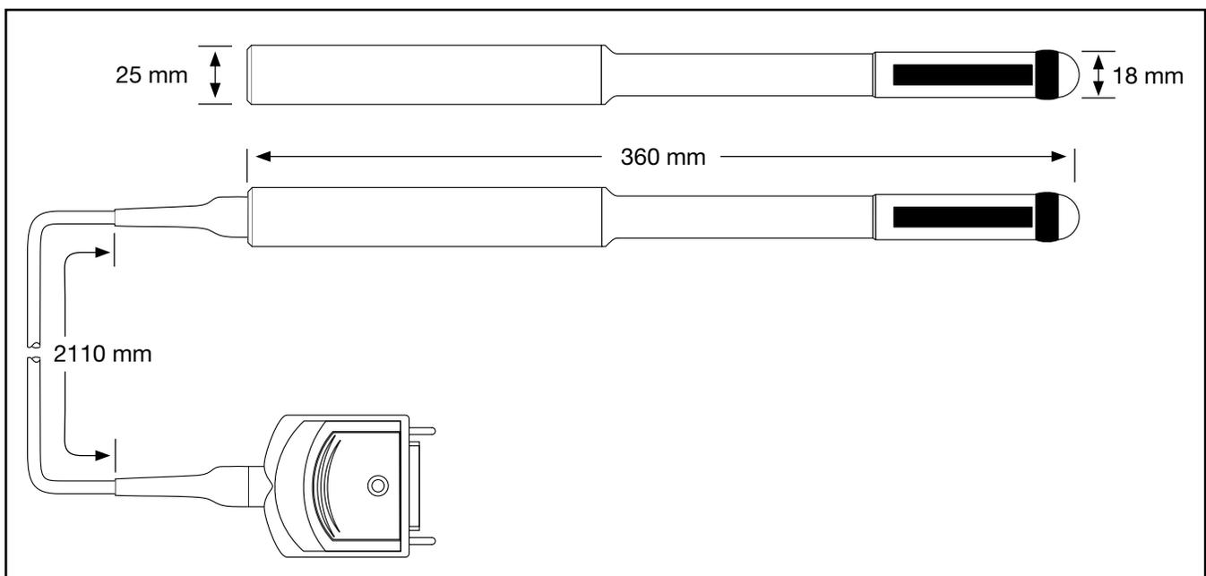
Figure 1-2: 8BP4 Probe with Measurements in mm
