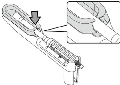
Example of storing a probe horizontally in a transvaginal/transrectal probe holder
