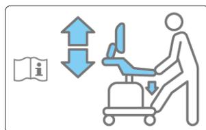
This label shows how to adjust the height of the operation panel.
