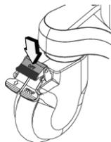
Step in the direction of the arrow to release the casters.
