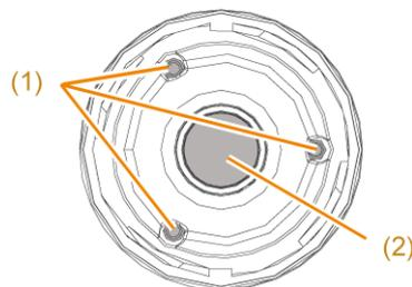
(1) Trackball support balls (2) Underside of the cup (the shadowed areas)
