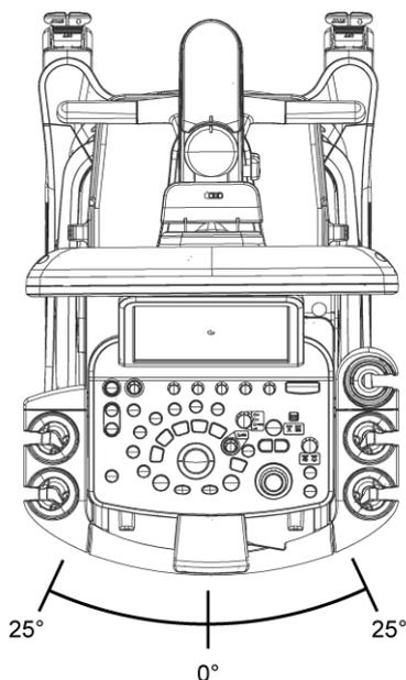
NOTE: Rotating the operation panel without holding the operation panel handle might damage the system.
