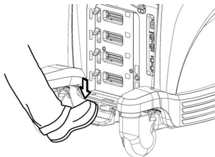
3. Release the up-and-down pedal of the operation panel to lock the height of the operation panel.
