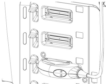
Example of connecting an electronic probe
