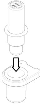
If the silicon rubber packing is difficult to insert
