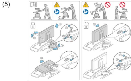
Follow the instructions in the manual to lock the monitor in position and to move the system.
