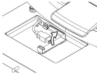
2. Connect the keyboard to the USB connector on the Keyboard Tray.
