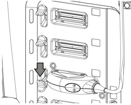
NOTE: Make sure the probe is secured.
