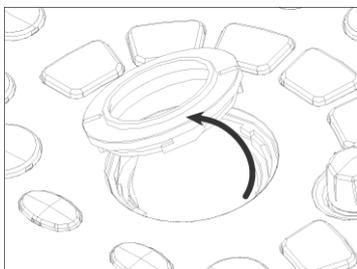
3. Remove the trackball from the operation panel and place it on a soft, lint-free cloth.
