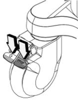
Step in the direction of the arrow to lock the casters.
