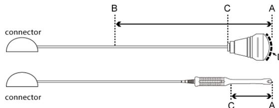
The upper figure is an example of a probe for body surfaces and intra-operative use. The lower figure is an example of a body cavity probe.
