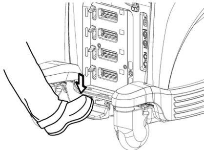
Press the operation panel height adjustment pedal
