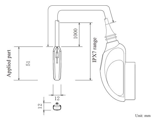
Remark: The tolerance for the dimensions is  $\pm 10\%$ .
