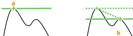
**a** Move the + mark to the first measurement point and tap the ultrasonic image area or select [Enter].
